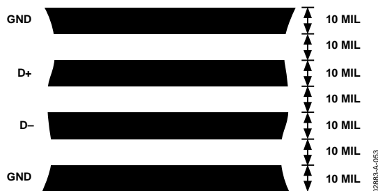
Figure 54. Arrangement of Signal Tracks
